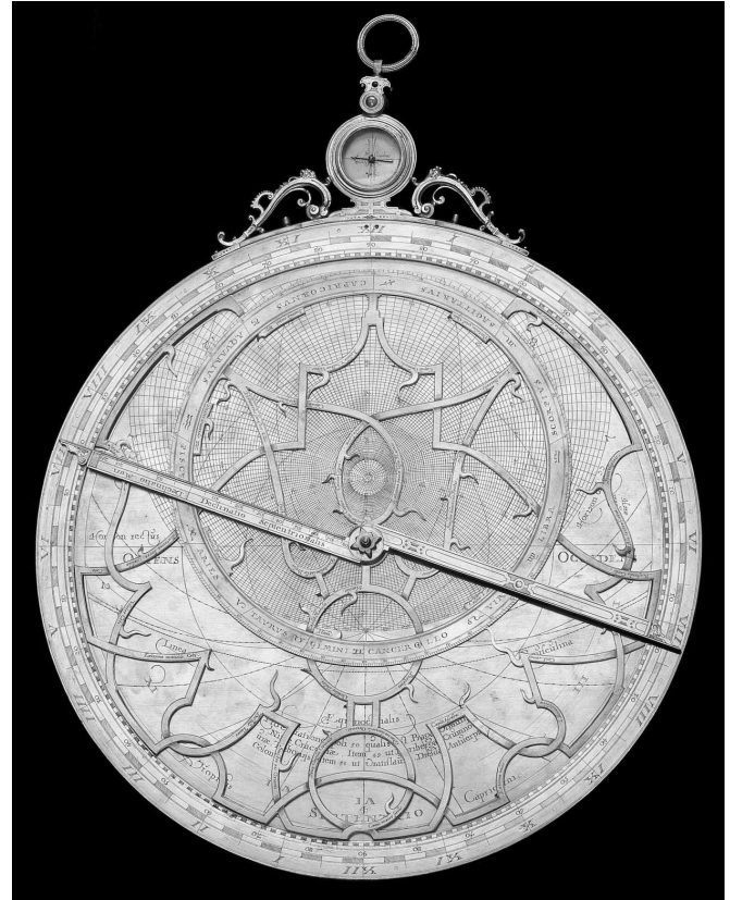
Fig. 6. Rule, ecliptic and time scales on the front of the astrolabe shown in Fig. 5.
