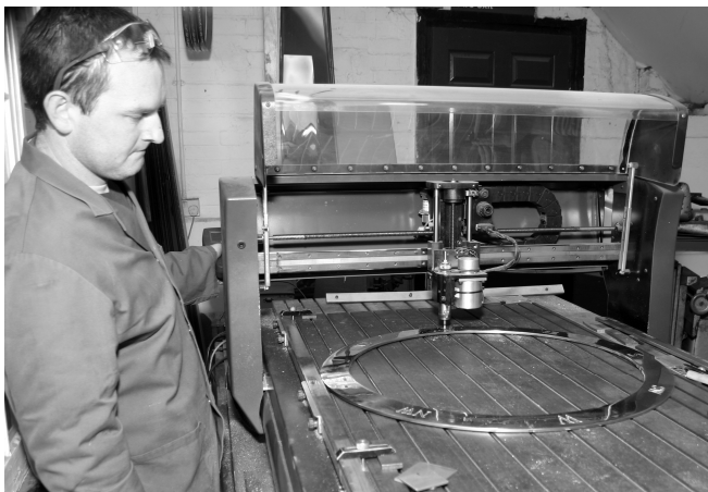
A flat bed computer controlled engraver.
