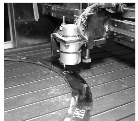
The engraver cutter working on a stainless steel armillary horizon ring.
