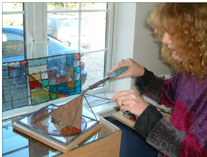
Fig. 2. The author soldering the gnomon into position with the aid of a temporary plywood jig.
