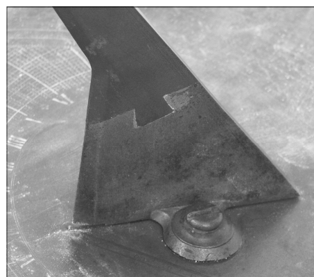
Fig. 8. Far left: a double horizontal dial and moon-dial by John Rowley. Left: Close-up of the repaired gnomon showing the original, slightly rough-textured, bottom section with integral feet.
