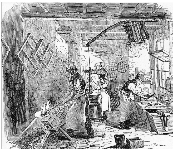
Fig. 3. Brass foundry work. This illustration from the London Illustrated News of 20 Sept 1851 shows the process at the clockmakers of J Smith & Sons, Clerkenwell. Brass ingots, smelted elsewhere, are melted and poured into moulds.
